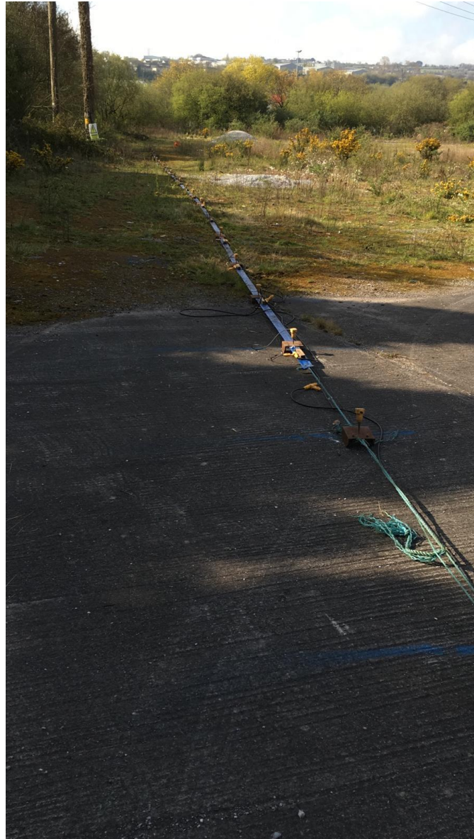
Figure C-1: MASW streamer in operation
